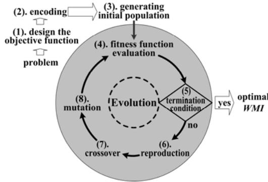
Figure 3. The GA flow chart for optimizing *WMI*.
