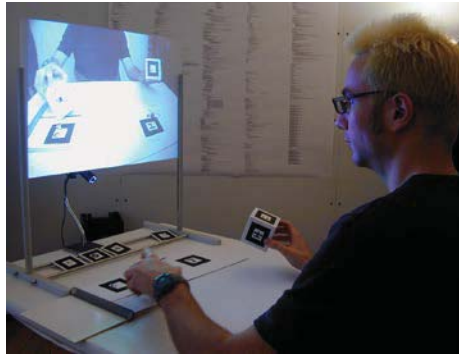
Figure 4. System set-up with a typical situation of use: charging the Gripper with an element from the booklet (left). The platform (right) holds an unsaturated atom, with which a binding with the charged atom may be triggered (Fjeld & Voegtli, 2002).
