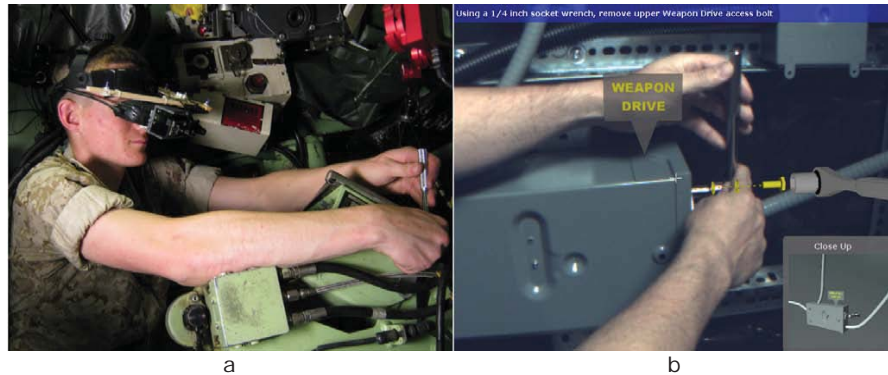
Figure 8. a) A mechanic wearing a tracked head-worn display performs a maintenance task inside an LAV-25A1 armored personnel carrier. b) The AR condition in the study: A view through the head-worn display captured in a similar domain depicts information provided using augmented reality to assist the mechanic (Henderson & Feiner, 2009).
