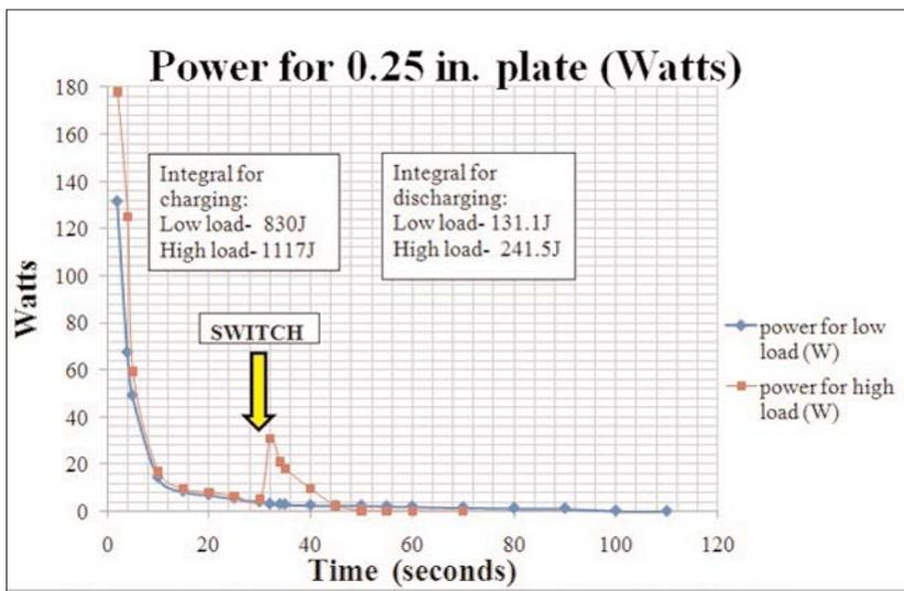
Figure 3 – Scatter plot of calculated power curve for low and high load for 0.25 in. plate
