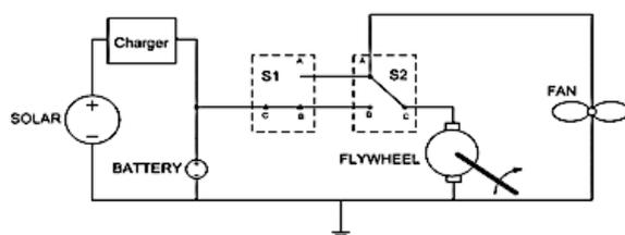
Figure 1 - Schematic Drawing of DC Load System
