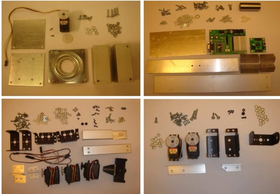
Upper left panel: The parts for the base. Upper right panel: The parts for the torso. Lower left panel: The parts for the arm. Lower right panel: The parts for the head.
