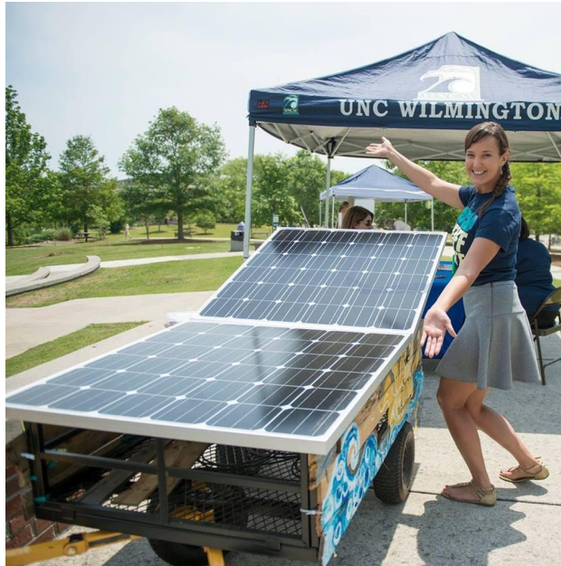
UNCW Sustainability Learning Community Solar Charging Station
