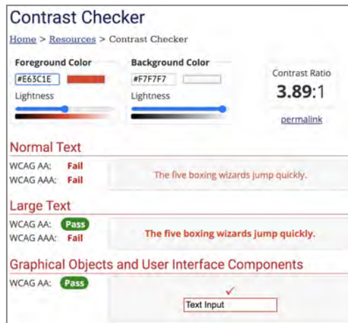
Figure 7. Color combinations from the red-templated web page from Figure 2 were analyzed with the WebAIM Color Contrast Checker. The resulting contrast was rated too low.
