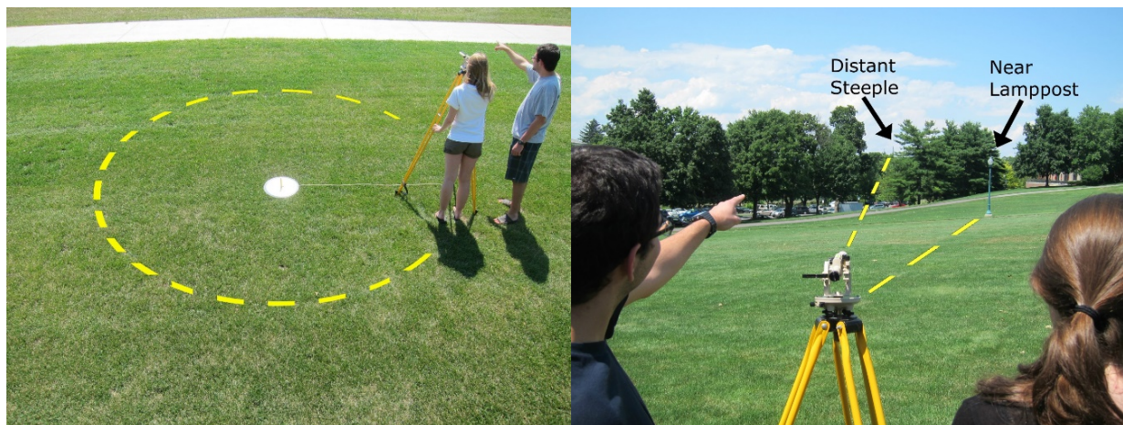
Figure 2. Students trace out a two-meter radius circle to mimic the Earth’s orbit around the Sun (left). Then they measure the direction to nearby objects from several locations along the circle. Using a surveyor’s transit, students measure the direction to a nearby lamp post, using the direction to a distant landmark as a reference (right).
