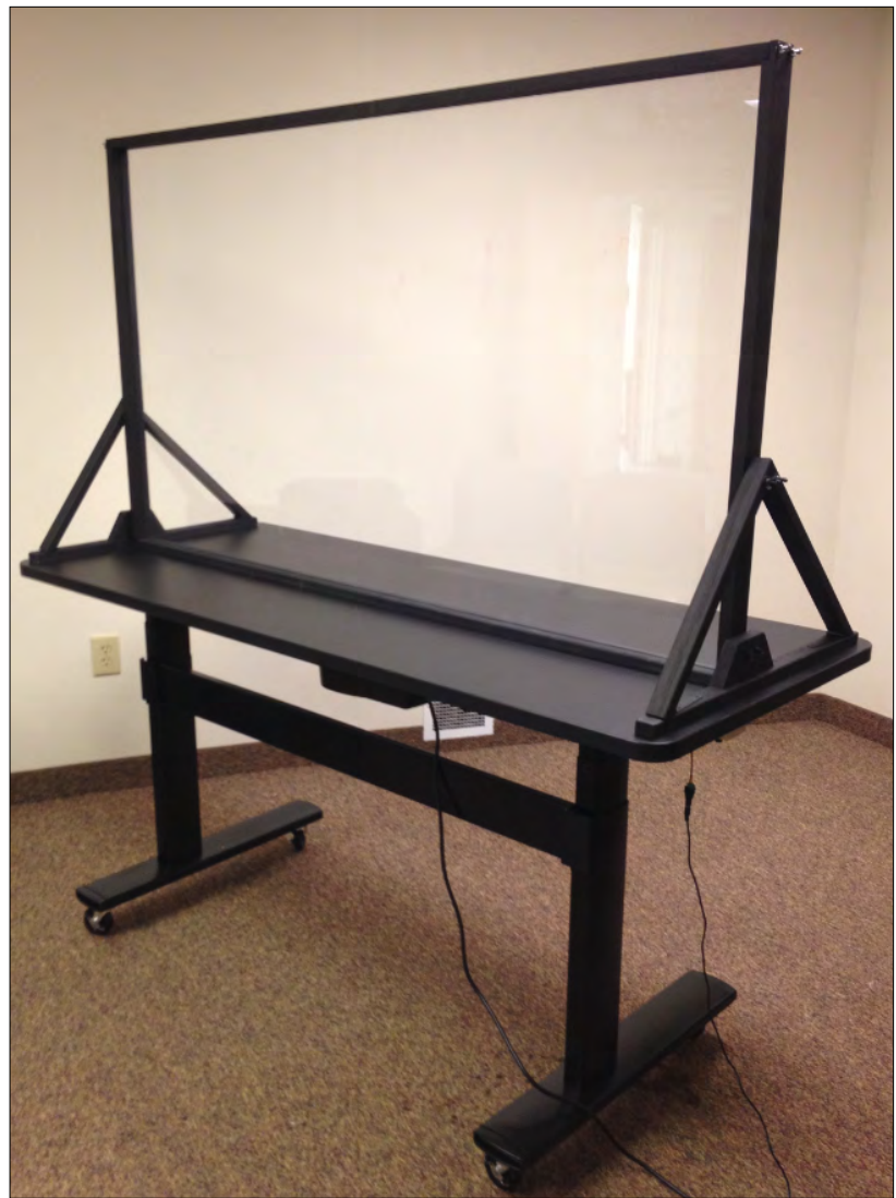
FIGURE 4. Full-scale Lightboard based on designs from Grand Valley State University eLearning and Emerging Technologies (n.d.) and the University of California San Diego (Anderson & Frazee, 2014) using Steelcase adjustable height tables. (Photo by Steven Wicker, Wake Forest University)
