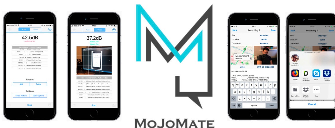
Figure 1. The mobile journalism machine assisted reporting platform (MoJo-MATE) terminal side. The mobile application contains modalities for the intelligent support of audio and video creation, as well as the sharing of the content along with automatically generated semantic annotation.
