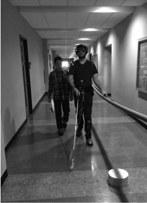
Figure 2. Participant approaching the obstacle on the obstacle detection path along the 20-foot-long guide rail.
