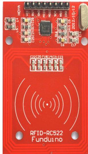
Figure 4. The RC522 module.
