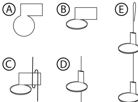
FIGURE 6. Fabrication of the double weighing pan. A) Cut out each pan from sheet metal, with a rectangular flange as shown. B) Bend the join between the pan and flange to a 90° angle. Press the round part over the end of a dowel, or similar tool, to create the shallow dish shape. C) Wrap a wire loop around the flange. D) Wrap the flange around the wire and crimp tightly. E) Repeat to make the lower pan. Trim the wire, leaving a loop at the top for a handle.
