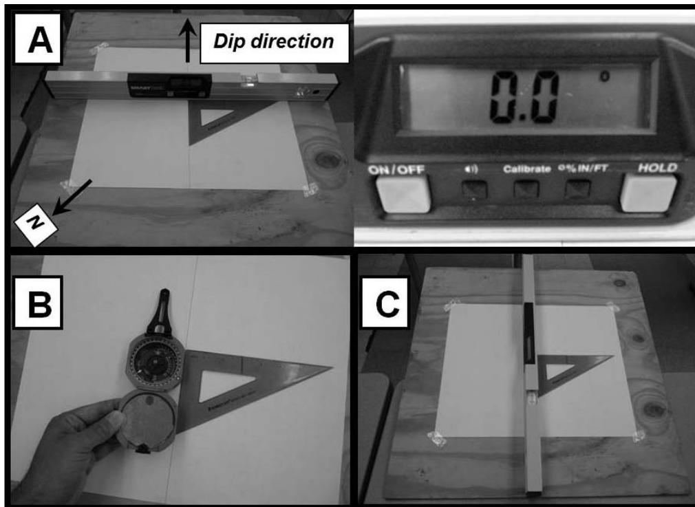
FIGURE 4: Measuring a bedding plane attitude with a digital level and a Brunton pocket transit. See text for more information. (A) Finding the strike. (B) Measuring the dip azimuth. (C) Measuring the dip.
