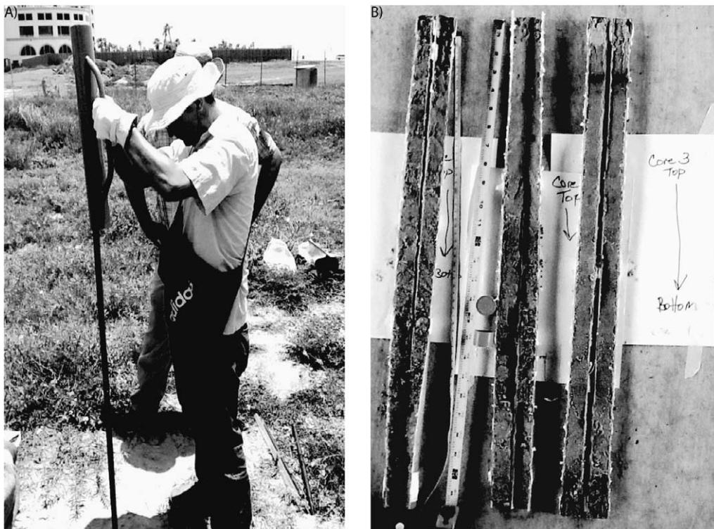
FIGURE 2: (A) Students had the ability to collect shallow sediment cores in a number of locations. (B) An example of three split sediment cores.
