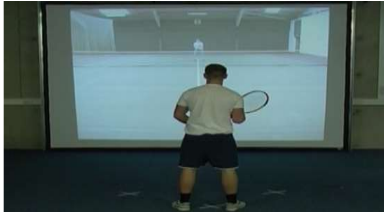
Figure 2. An illustration of a film-based simulation used to evaluate anticipation and decision making in tennis. The participant is required to anticipate the location and type of shot played by the opponent located at the net and to decide on an appropriate response. Verbal or motor responses are recorded (both speed and accuracy), with the latter from pressure sensitive mats placed on the floor around the participant.
