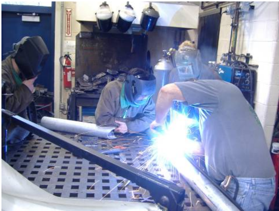
Figure 2. One of the authors assists a group students welding a crossbeam for a handicap accessible swing set
