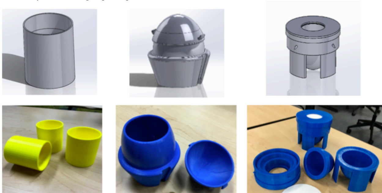
Figure 1. Computer aided drawings and 3d-printed prototypes for several egg incubation vessels that were designed, fabricated and tested by Madison College engineering students for stem cell research
