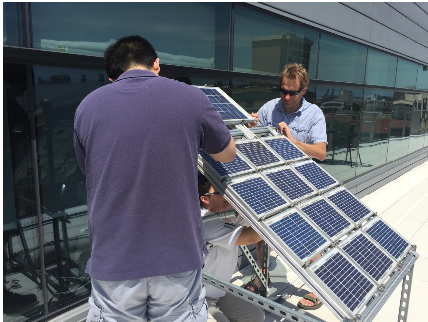
Figure 3. One of the authors works with a UW graduate student on a photovoltaic panel test apparatus, designed and fabricated by undergraduate engineering students at Madison College.
