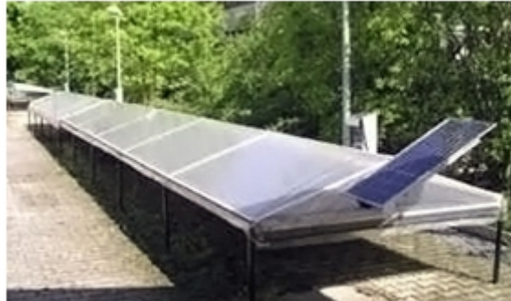
Figure 6. AlgaeLink solar dryer for microalgae (AlgaeLink, 2015)
