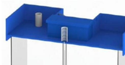
Figure 10. The fail-safe stand pipe
