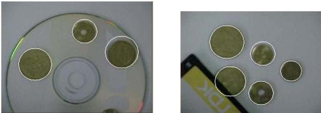
*Figure 2. Two examples of the results of the lab assignment: counting coins. The white circumferences are the coins detected. Note that the CD is not detected as it has a different colour, and the inner circle of several coins is not detected either*
