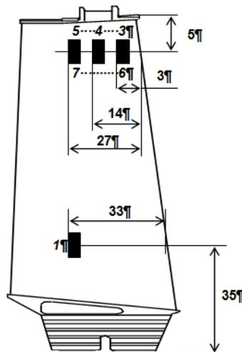
**Figure 2.** Comparison of the calculated and measured stress in the cooled working blade during tests on acceleration bench. Strain sensors 1, 3, 4, 5 are located on suction side; strain sensors 6 and 7 - on the pressure side.
