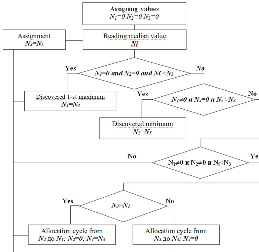
**Figure 5.** Flowchart of the algorithm for distinguishing “simple” cycles
