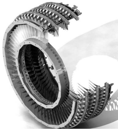
Figure 1. The physical form of a VGV of three compressor stages
