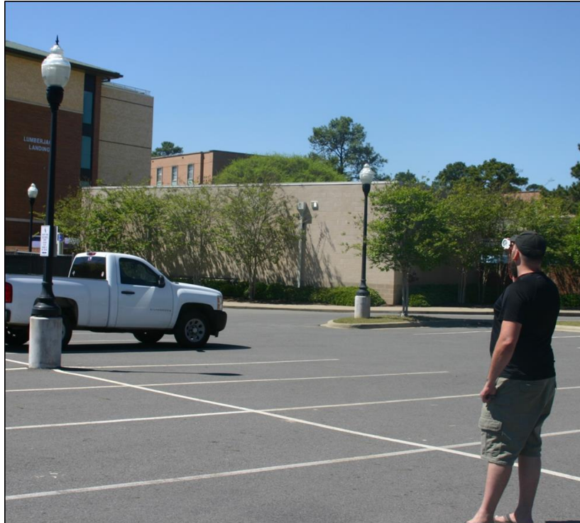
Figure 4. Estimating in situ height with a clinometer
