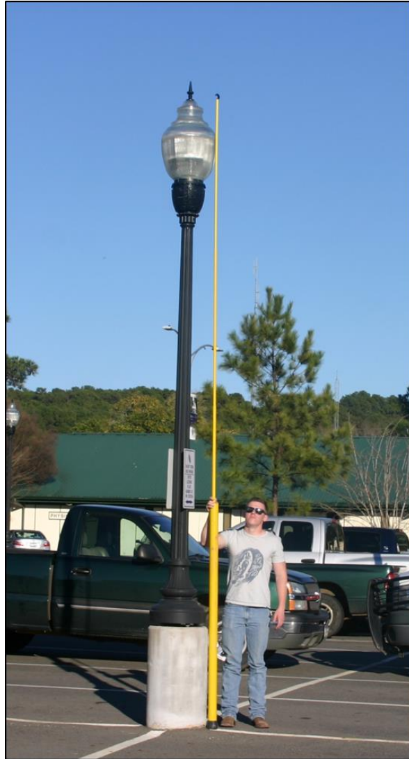
Figure 3. Measuring in situ height with a telescopic height pole
