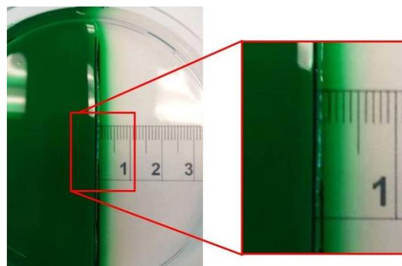
**Figure 4.** Representative image of gel after 120 minutes. By this point, the green dye has diffused into the gel several millimeters. The enlarged image at right illustrates how the leading edge of the dye is not sharply delineated. Each group of students is asked to discuss where they believe the leading edge is located and then reach a consensus measurement. This variability provides a point of discussion when compared to the model.
