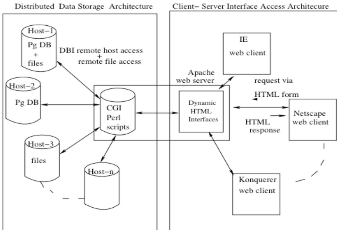
**Figure 1:** Architecture of WBCM package
