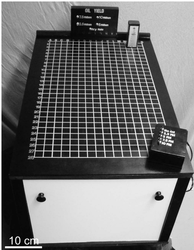
FIGURE 2: The oil game model showing a gridded top for drill locations, a derrick to mark well locations, and a light-buzzer board on the rear (oil yield), with the control box in front. The white panel with knobs conceals the geology.
