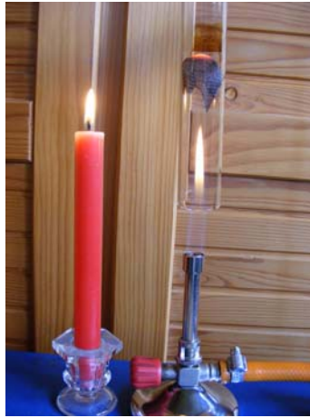
Picture 4. Threshold-effect in the heat power: in case of a too low power input (candle light) none of the tubes issued any sound, but just a little bit bigger power input (gas-jet) was enough to generate sound
