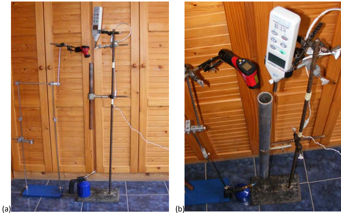
Picture 1. Vertical Rijke pipe with measuring arrangement (a) copper tube; (b) shorter aluminium tube
