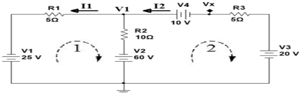
Figure 14. Equivalent Circuit To That Shown In Figure 11
