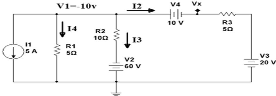
Figure 12. Equivalent Circuit To That Shown In Figure 11
