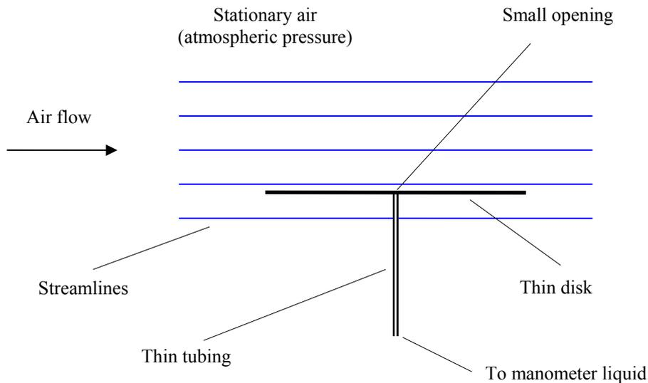
Figure 2. Using a manometer to measure static pressure.
