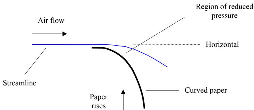
*Figure 1.* Blowing air across the top of a curved object.
