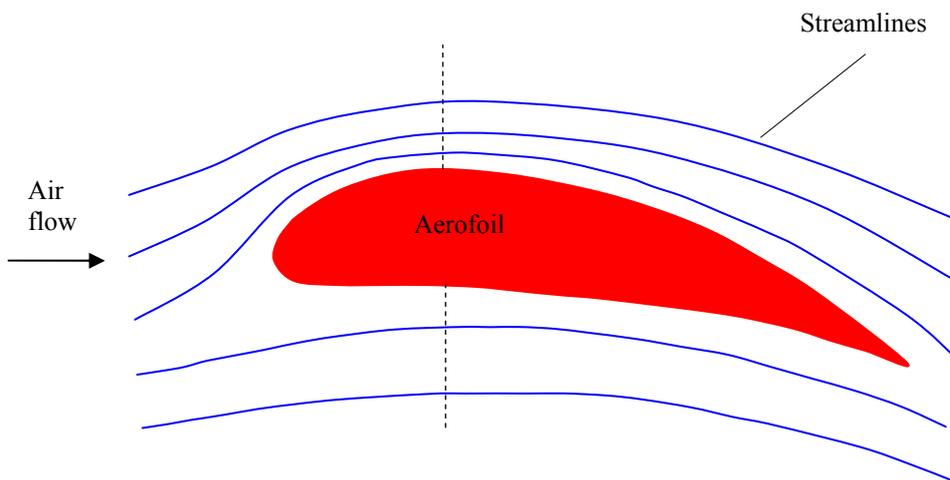
Figure 4. General pattern of streamlines around an aerofoil.
