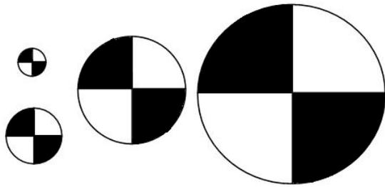
**Fig. 2.** Mini-Secchi discs. Discs pictured are 10 mm, 15 mm, 35 mm, and 55 mm in diameter. Students should use the smallest possible disc for the experiment. Photo-reduction can also be used to adjust disc size as needed.
