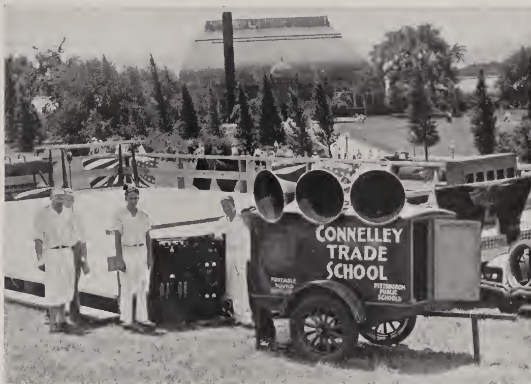
Sound Amplifier Constructed by Clifford Connelly Trade School Students.
