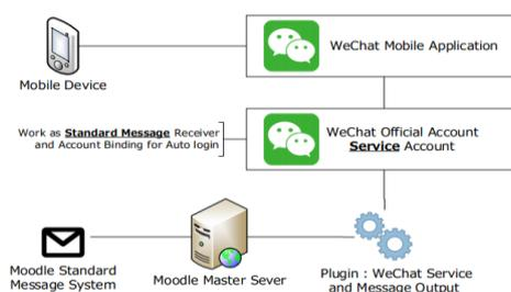
Figure 2. The basic structure of advanced integration
