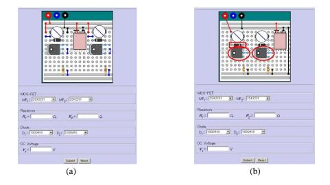
Figure 4. Circuits of line tracers constructed by two students using the VCM function: (a) correct circuit and (b) incorrect circuit and automated indication of incorrect parts.
