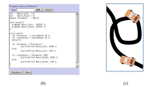
Figure 5. Results of the virtual construction and simulation of the circuit of a line-tracer robot: (a) virtual circuit of a line tracer constructed using the VCM function, (b) Arduino program written by the student, and (c) one frame that was captured from the simulated moving image based on Program (b).
