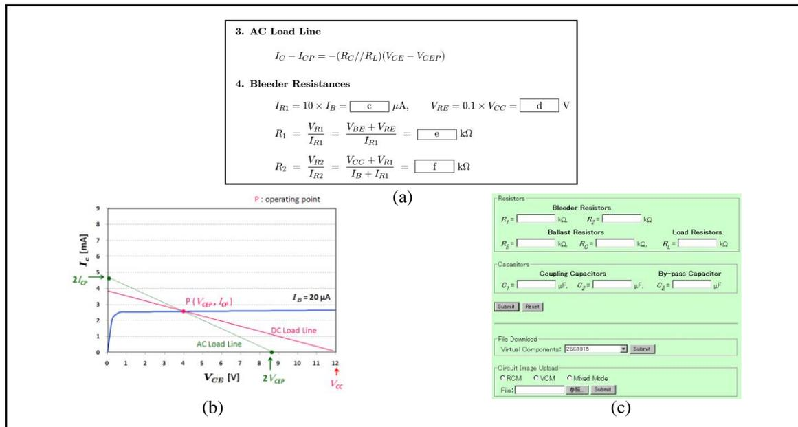
Figure 4. (a) Operating point and load lines that are indicated on  $V_{CE}$ - $I_C$  characteristics, (b) manual to calculate the circuit parameters, and (c) input forms to submit the information of the designed circuit.
