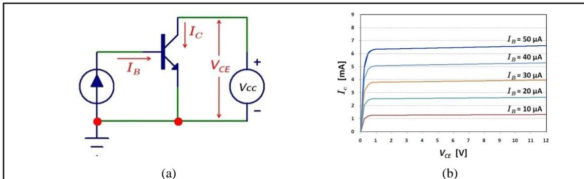
Figure 2. Static characteristics of an amplifier with a transistor; (a) circuit diagram, and (b)  $V_{CE}$ - $I_C$  characteristics.
