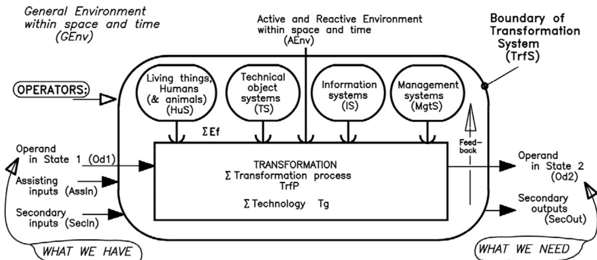
Figure 7. General model of a transformation system. Source: Eder and Hosnedl (2008; 2010).
