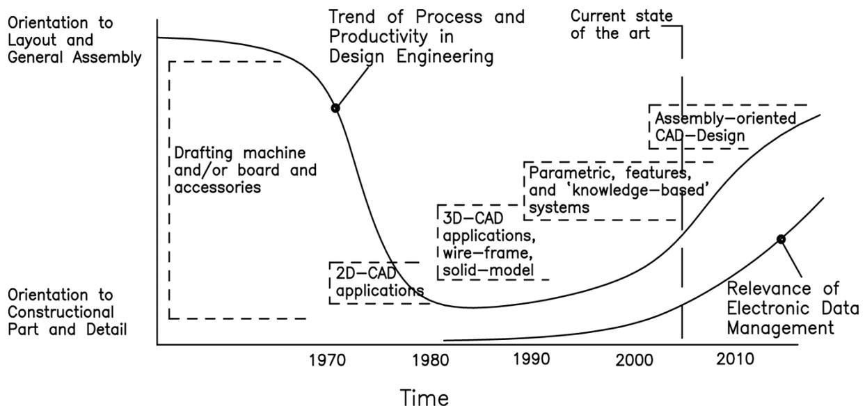
Figure 13. Progress of computer support of representation for design engineering. Source: Eder and Hosnedl (2008, 2010; as cited in Burr et al., 2005, with permission).
