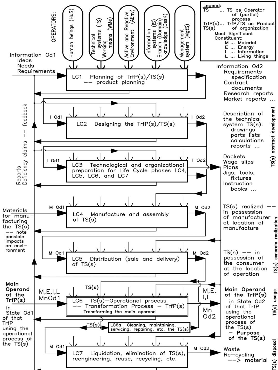
Figure 8. Typical life cycle of a TS. Source: Eder and Hosnedl (2008).
