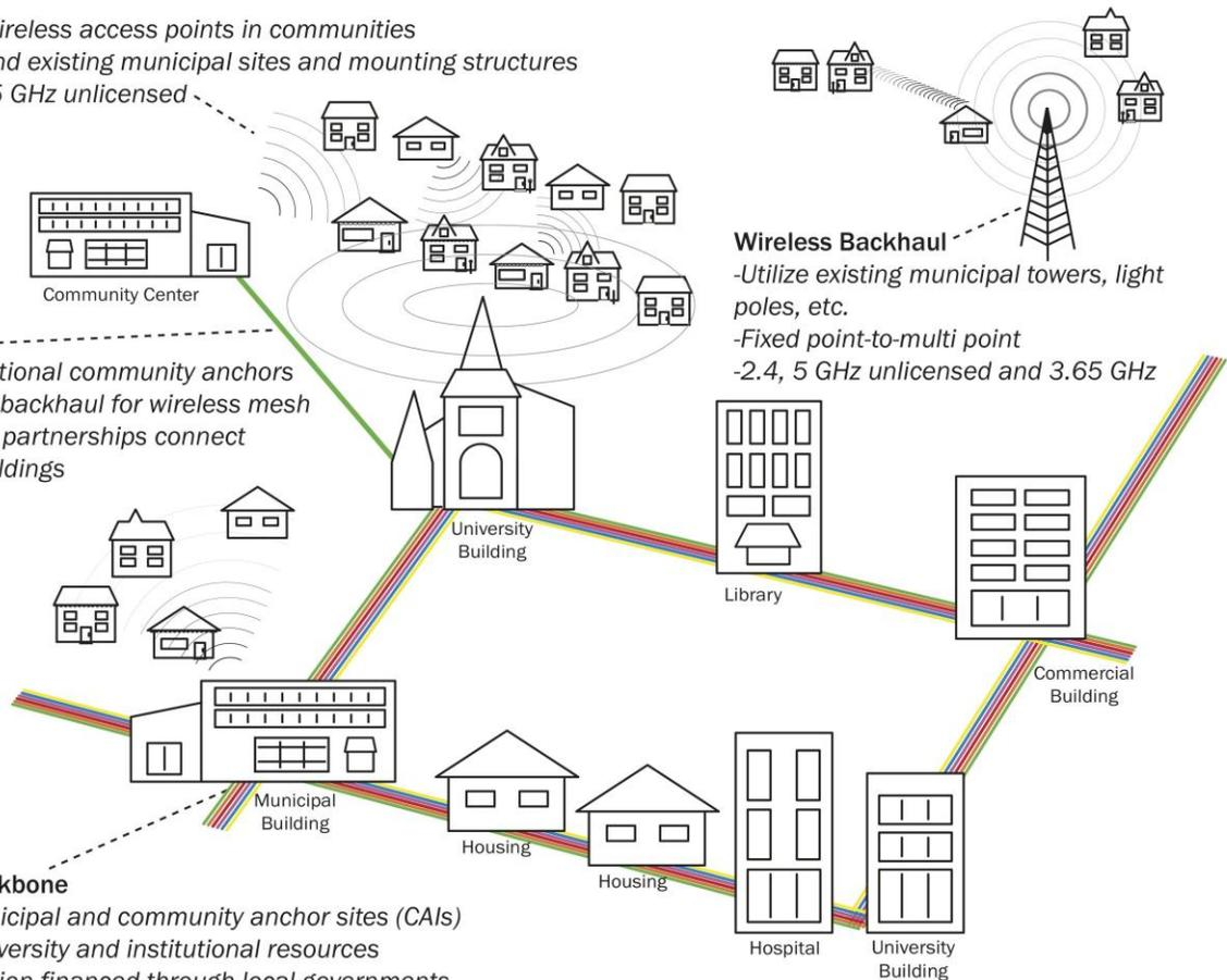
Figure 1: Example of Fiber and Mesh Wireless Network
