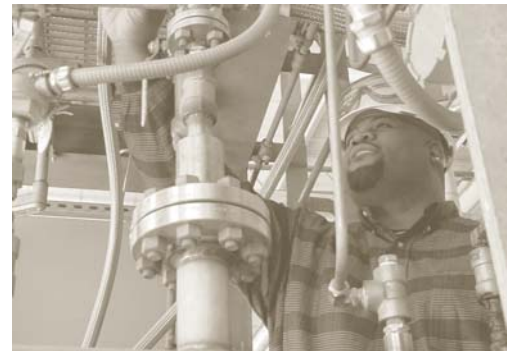
Carl Ilks, a process technology student, monitors and adjusts vacuum pressure on the Glycol Separation Training Unit at the College of the Mainland in Texas City, Texas, home of the Center for the Advancement of Process Technology.
