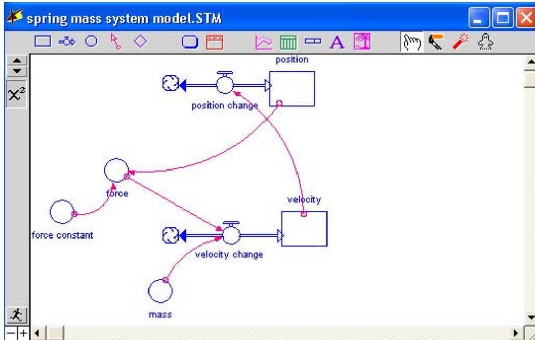
**Figure 3.** Modeling To Spring Mass System with Stella
