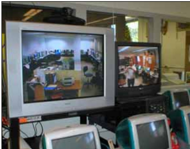
Videoconferencing courses often use two television monitors to display each participating site. They also use a digital camera and speakers, shown on top of the larger screen.
