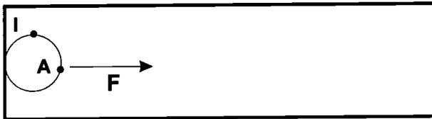
**FIGURE 1.** A puck on a horizontal frictionless table; a constant force is applied always at the same point, either A (case a) or I (case b).
