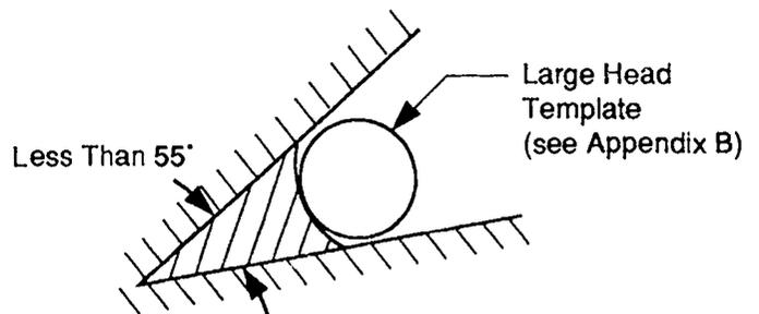
**Figure 5 Shield for Angle Less than 55°**
