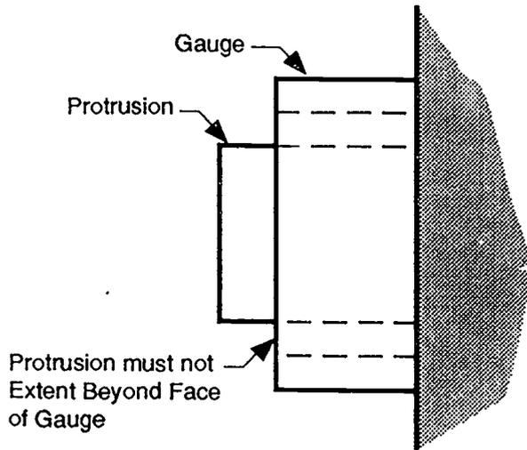
Figure 2 Protrusion Test
