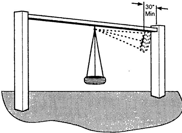
**Figure 11 Multi-Axis Tire Swing Clearance**
