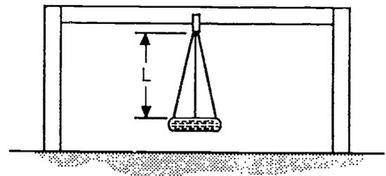
Figure 18 Fall Zone for Multi Axis Tire Swings
