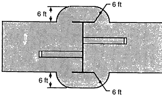
Figure 17 Fall Zone for Single Axis Swings
