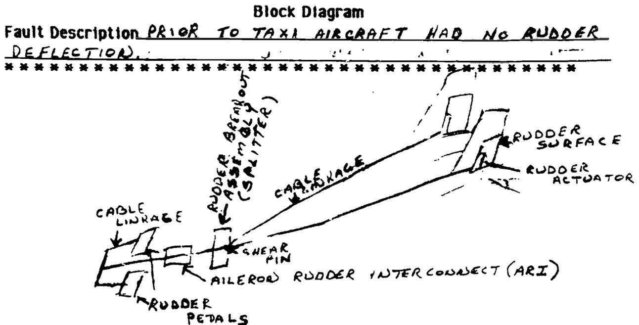
Figure 1. SME Block Diagram
