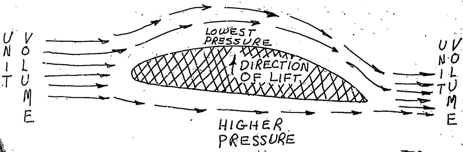
**FIGURE 4. A Fluid Passing Over An Object With One Surface Having A Greater Curve Than The Other**
