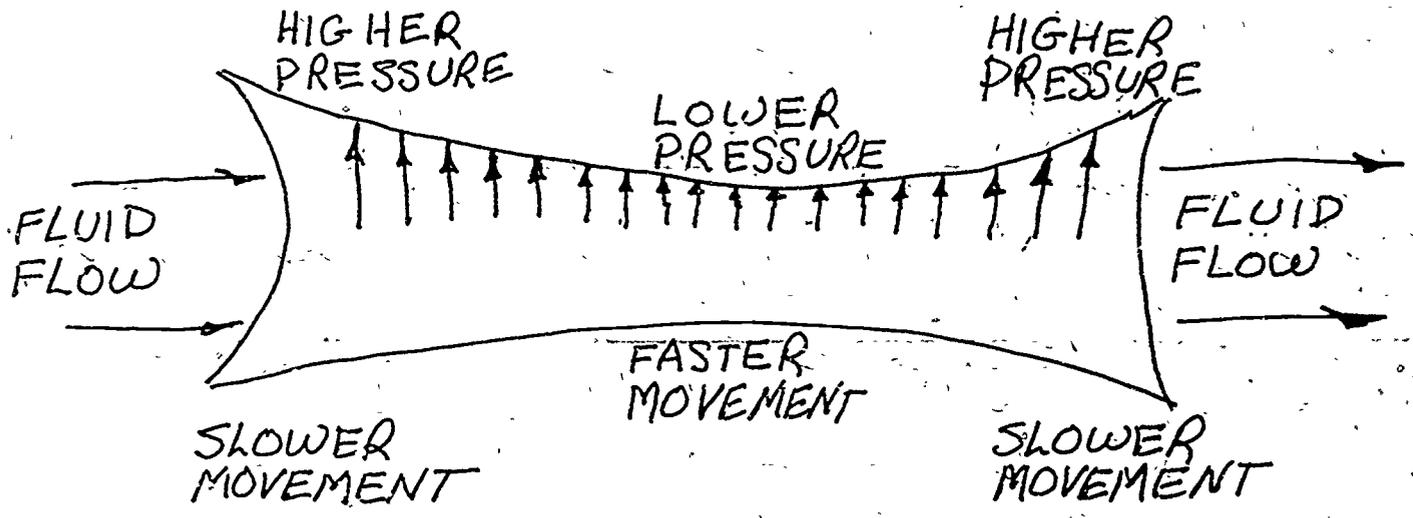
**FIGURE 3. Arrow Vectors Showing Differential Pressure Exerted On the Sides Of A Constricted Area By A Fluid.**
