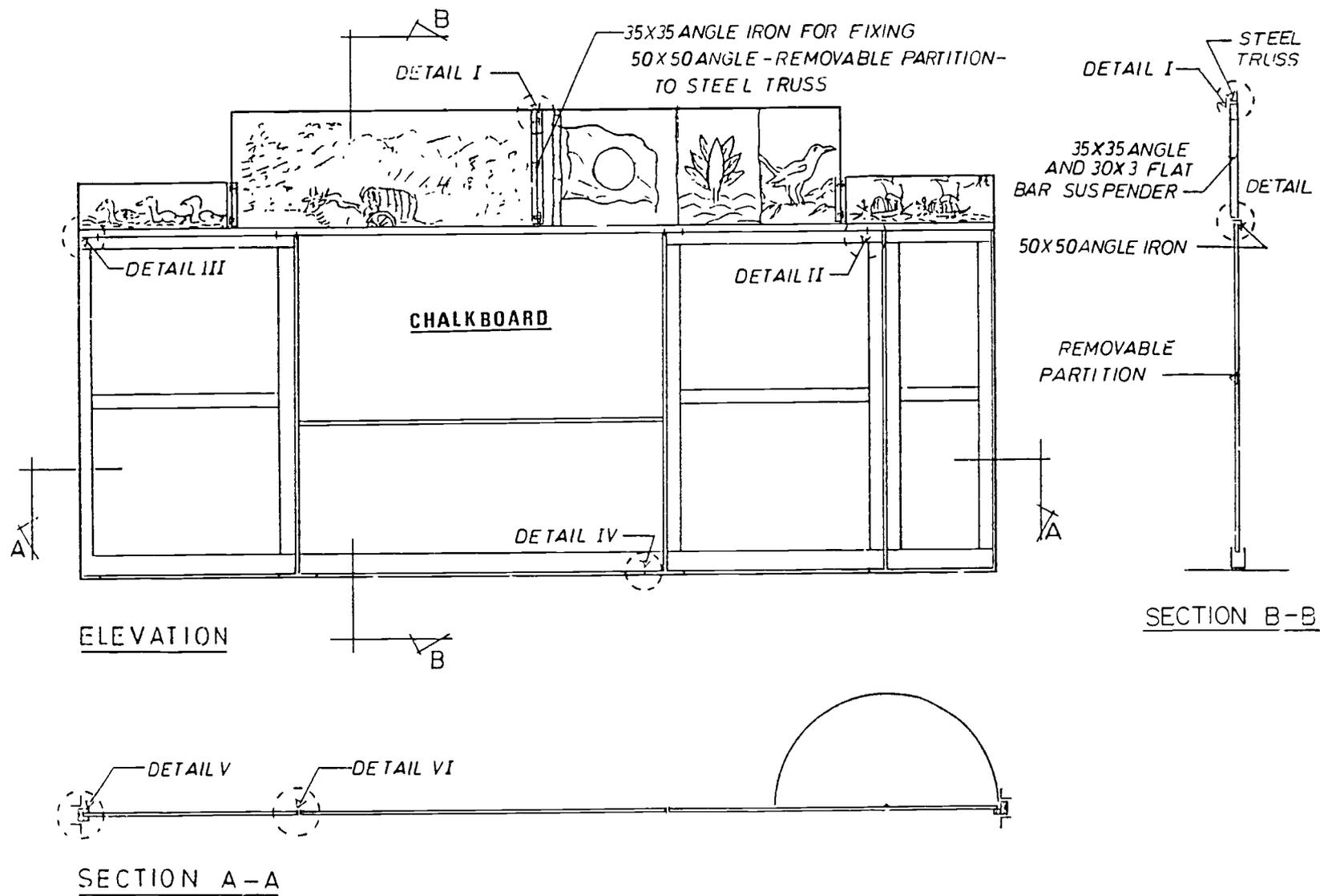
**FIGURE 16 REMOVABLE PARTITION - FIXING DETAILS**
