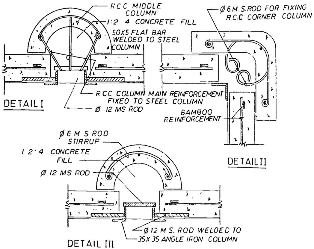
**FIGURE 8 CASTING OF R.C.C. PREFAB COLUMNS**
