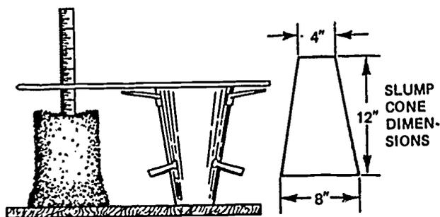
Fig. 4-2. Measuring concrete slump
