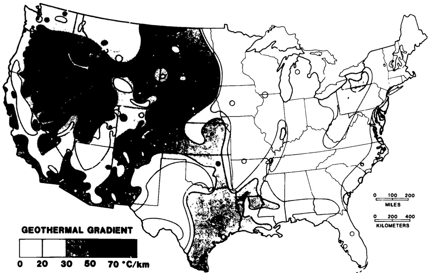
**Geothermal gradient map of the United States based on gradients measured where the terrestrial heat flow is by conduction through the rock.
