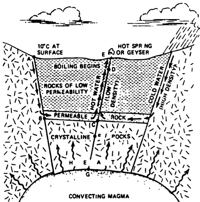
Diagram of a geothermal reservoir. Source: "Sourcebook on the Production of Electricity From Geothermal Energy" U.S. Department of Energy
