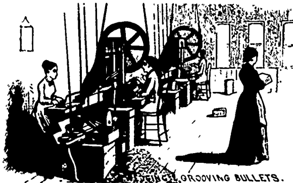
WEDGING AND GROOVING BULLETS. Wedging and grooving bullets at Remington & Sons, Ilion, New York. From Scientific American 45 (1881), p. 143.
