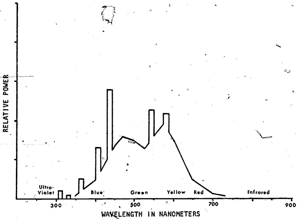
Figure 4. Spectrum of full-spectrum (daylight) fluorescent lamps.
