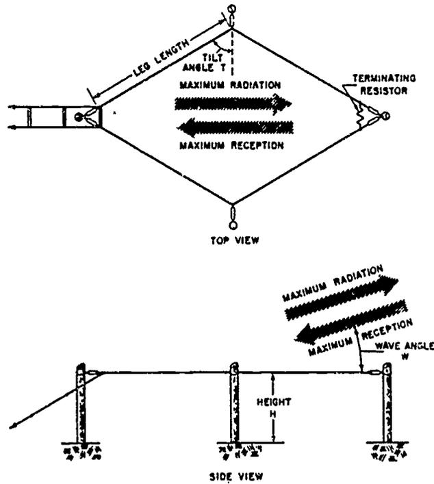
Fig 4-11. Basic rhombic antenna.
