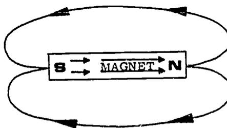
Fig 1-7. Lines of force in a bar magnet.
