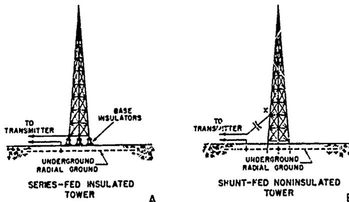
Fig 3-13. Series- and shunt-fed tower radiators.
