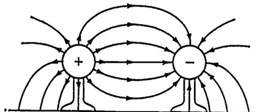
Fig 1-3. Direction of electric field about positive and negative charges.
