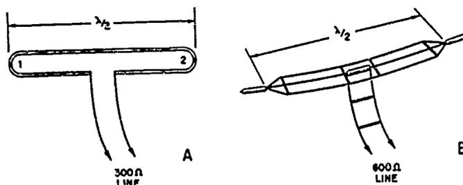
Fig 3-22. Folded-dipole antenna.
