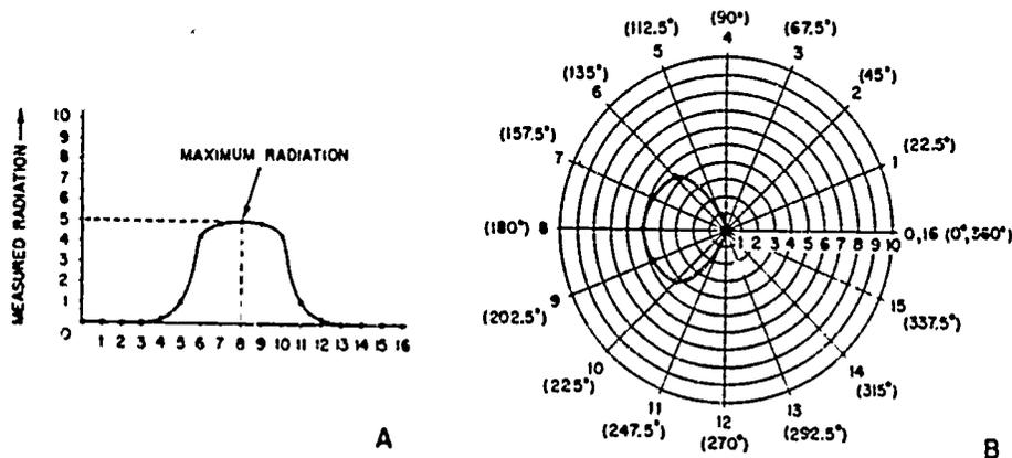
Fig 2-17. Comparison of rectangular- and polar-coordinate graphs for anisotropic source.
