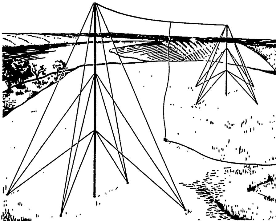
Fig 3-21. Single-wire antenna.
