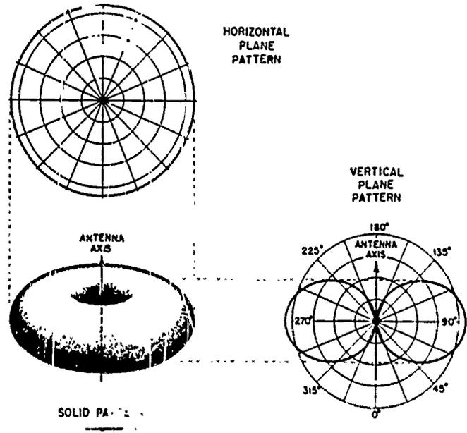
Fig 3-15. Radiation pattern of a dipole (half-wave) antenna.
