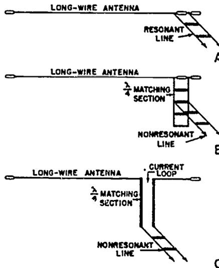
Fig 4-3. Feeding long-wire antennas.
