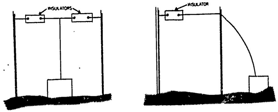
Fig 3-7. Bent antennas (T Bent, L Bent).
