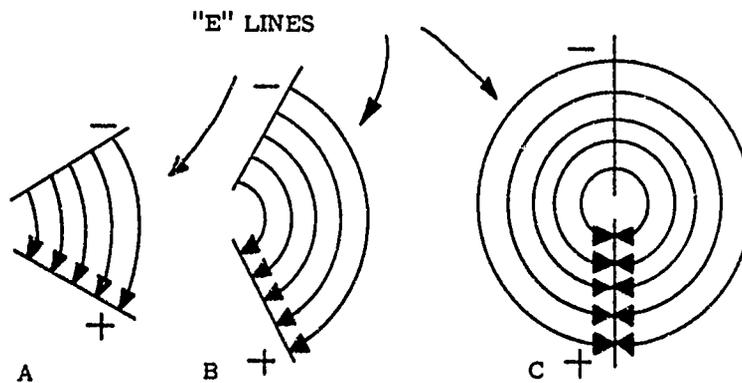
Fig 2-6. Open electric field.
