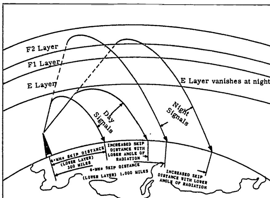
Fig 5-20. Relationship between distance, time, angle, and frequency.
