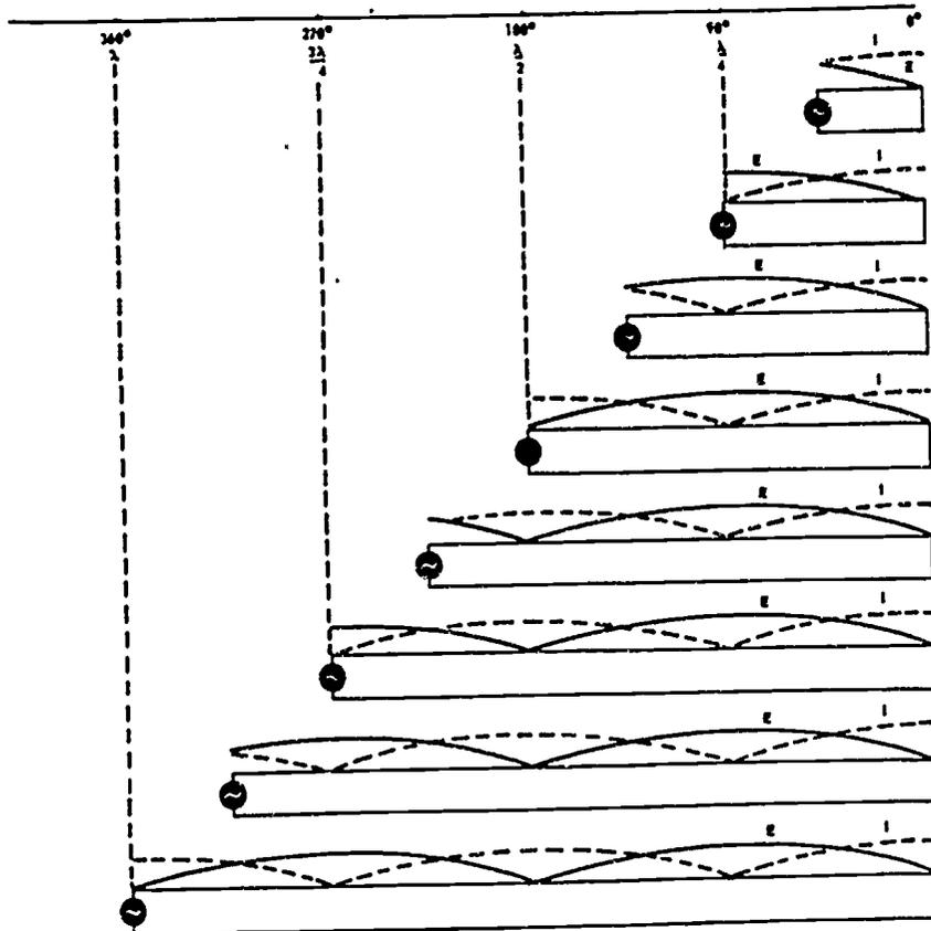
Fig 2-22. Voltage and current on a shorted transmission line.
