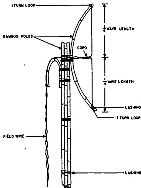
Fig 4-26. Improved method of supporting a vertical half-wave antenna.
