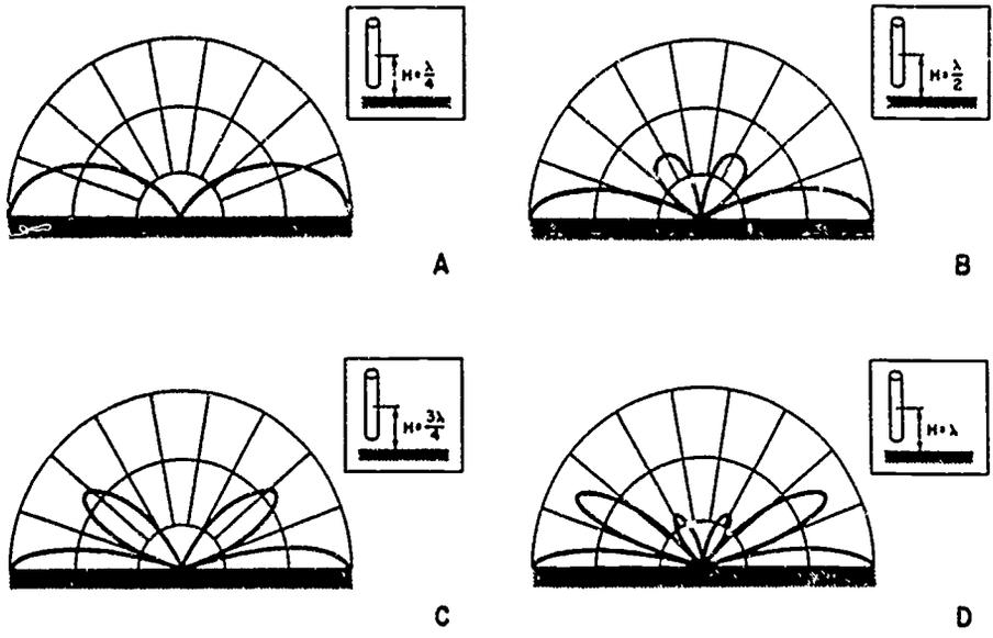
Fig 3-19. Vertical-plane radiation patterns produced by vertical half-wave antennas.
