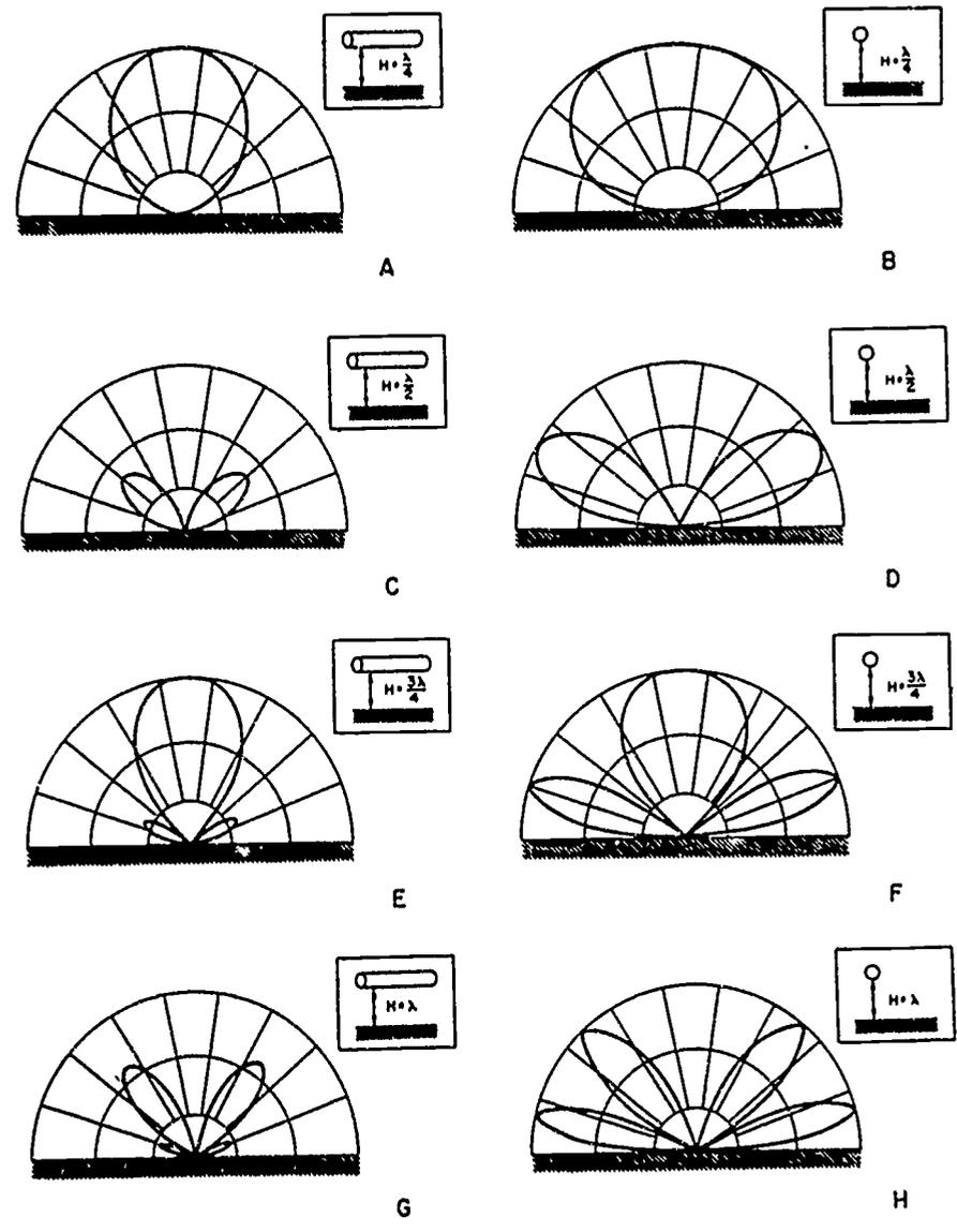
Fig 3-17. Vertical-plane radiation patterns of horizontal half-wave antennas.
