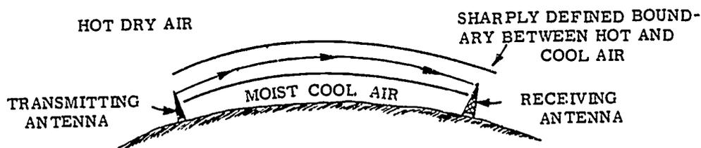
Fig 5-9. Transmission using the tropospheric duct.
