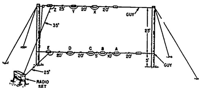
Fig 3-8. Inverted-L antenna with counterpoise.
