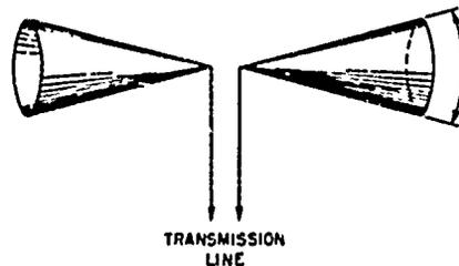
Fig 3-24. Simplified conical antenna.
