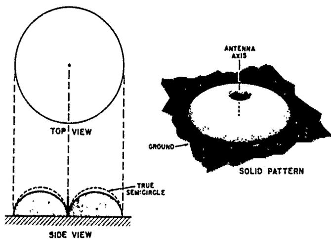
Fig 3-3. Radiation pattern of a quarter-wave antenna.
