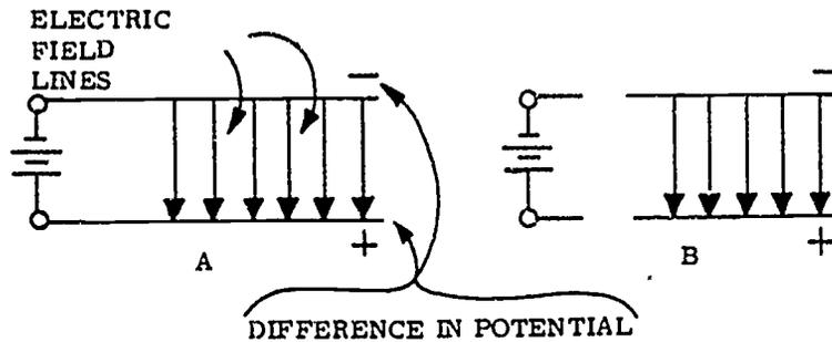
Fig 2-5. Electric field between capacitor plates.
