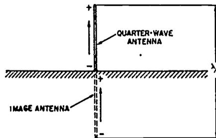
Fig 3-1. Quarter-wave antenna connected to ground.
