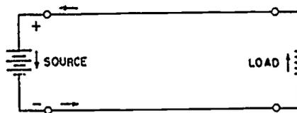
Fig 1-5. Current (electron) flow in a circuit.
