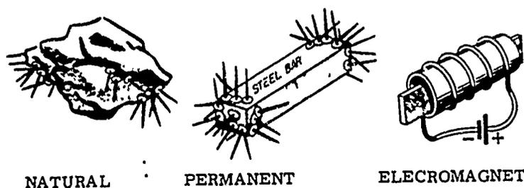
Fig 1-8. Three types of magnets.
