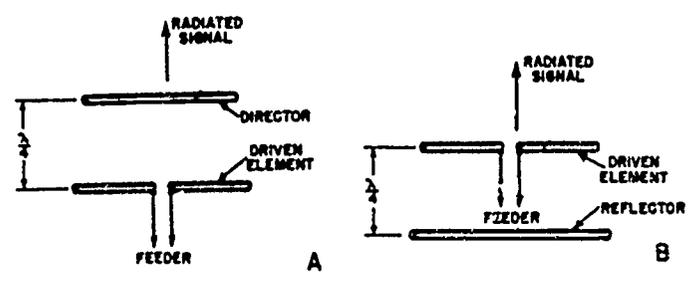
Fig 3-27. Position of the director and reflector to the driven element.
