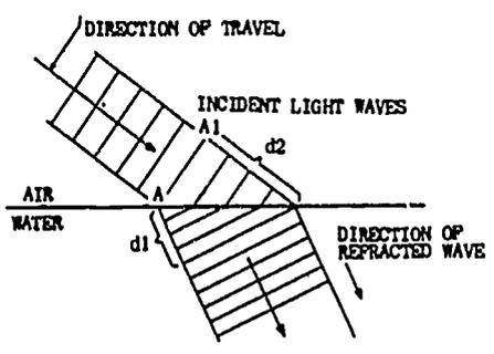
Fig 5-4. Refraction.
