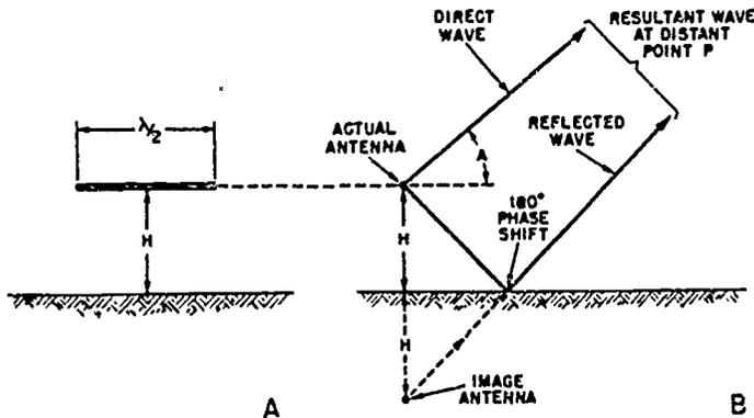
Fig 3-16. Reflection produced by ground plane.
