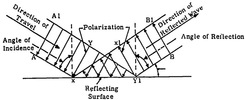
Fig 5-2. Reflection of a radio wave.
