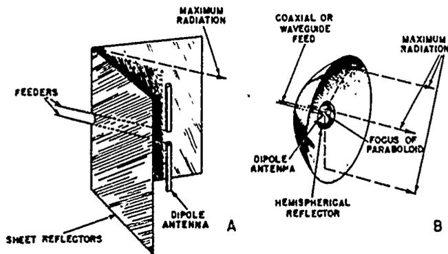
Fig 3-26. Special reflectors for half-wave antennas.
