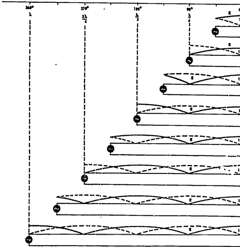
Fig 2-21. Voltage and current on an open transmission line.
