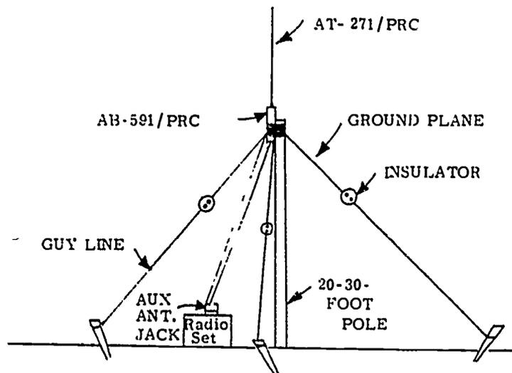
Fig 4-29. Ground plane antenna improvised by using the AN/PRC-25 antenna.
