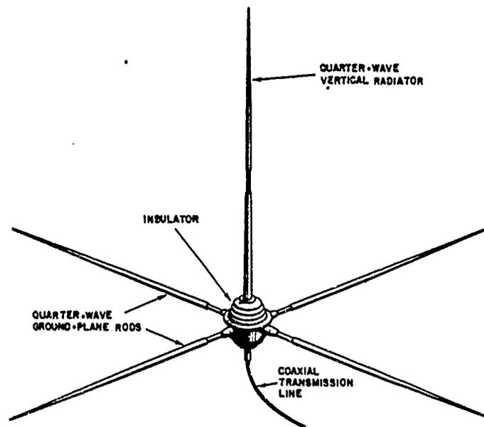
Fig 3-5. Typical ground plane antenna.
