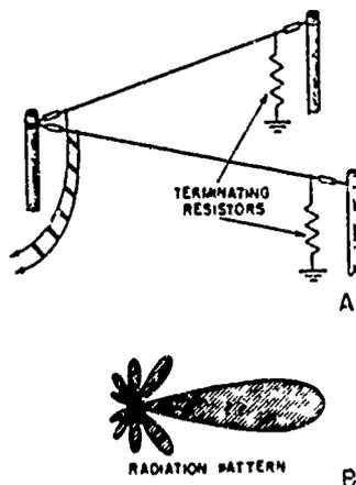
Fig 4-7. Unidirectional V antenna.
