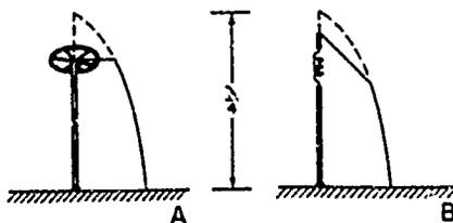
Fig 3-11. Top-loaded antennas.
