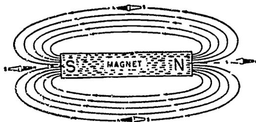
Fig 1-11. Magnetic lines of force.
