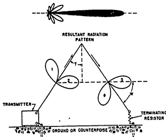
Fig 4-10. Terminated half-rhombic antenna and resultant radiation pattern.
