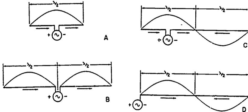
Fig 4-1. Harmonically and nonharmonically operated antennas.
