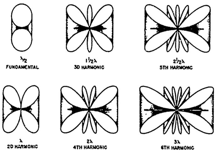
Fig 4-2. Radiation patterns of various harmonic antennas.
