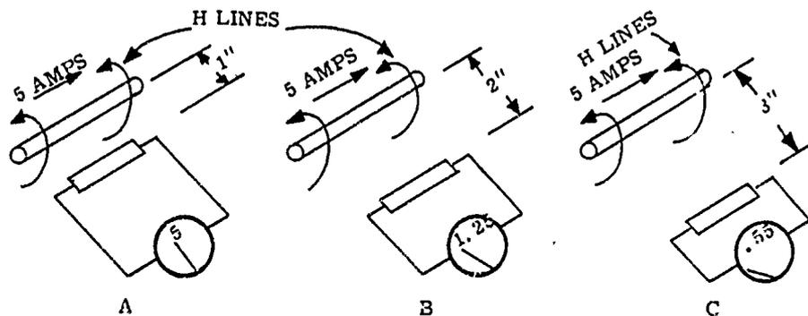
Fig 2-4. Effects on the "H" field as the distance from the conductor is varied.
