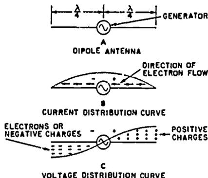
Fig 2-10. Voltage and current distribution of a dipole antenna.
