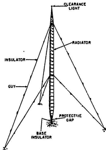
Fig 3-12. Insulated guyed-tower radiator.
