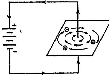
Fig 2-1. Magnetic field about a current-carrying conductor.
