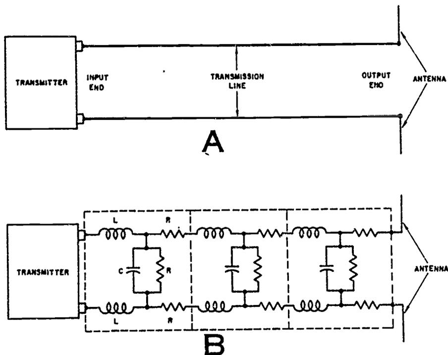
Fig 2-20. A transmission line and its equivalent circuit.
