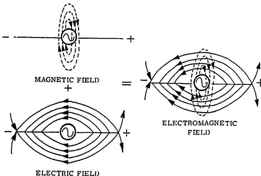
Fig 2-8. Components of the electromagnetic field.
