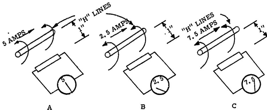
Fig 2-3. Effects on the "H" field as current through the conductor is varied.
