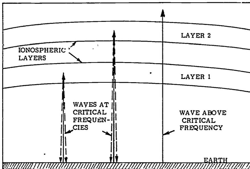
Fig 5-12. Critical frequencies in relation to waves.
