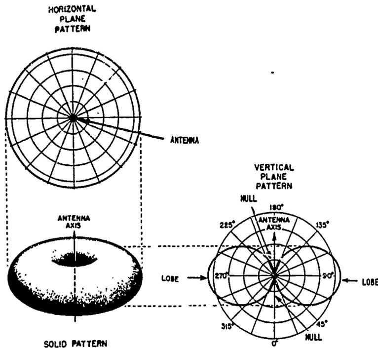
Fig 2-18. Radiation pattern of a dipole antenna.
