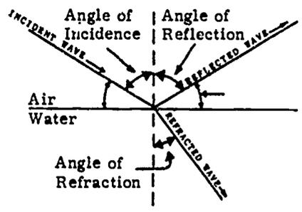
Fig 5-3. Reflection and refraction.
