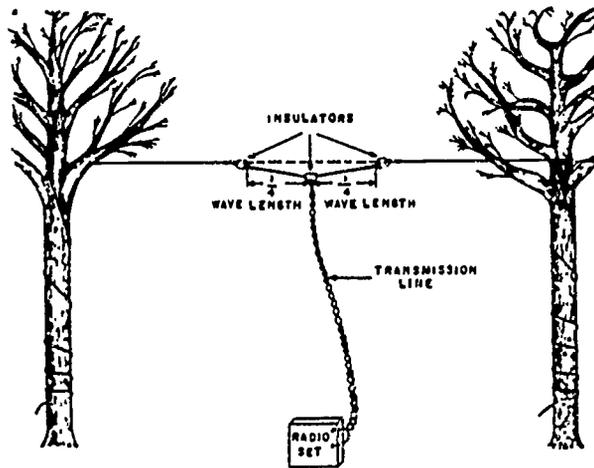
Fig 4-24. Improvised half-wave antenna.
