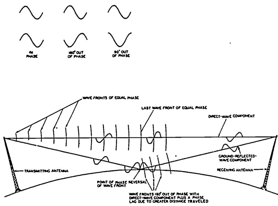
Fig 5-7. Comparison of the direct and the ground-reflected wave.
