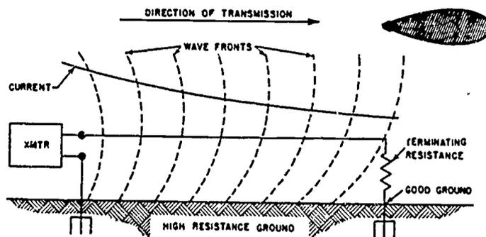
Fig 4-4. Beverage or wave antenna.
