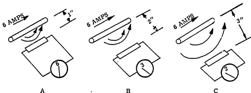
Fig 2-7. Effects on the "E" field as the distance from the conductor is varied.
