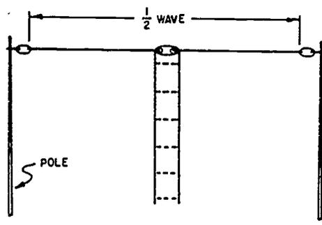
Fig 3-14. Basic Hertz antenna.
