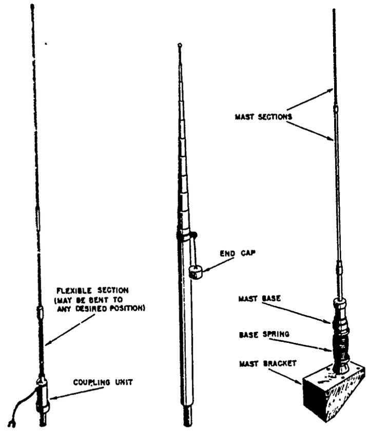
Fig 3-4. Common quarter-wave whip antennas.
