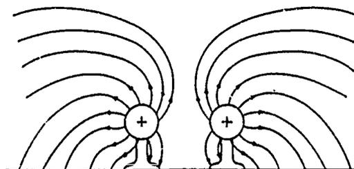
Fig 1-4. Electric field between two positively charged bodies.
