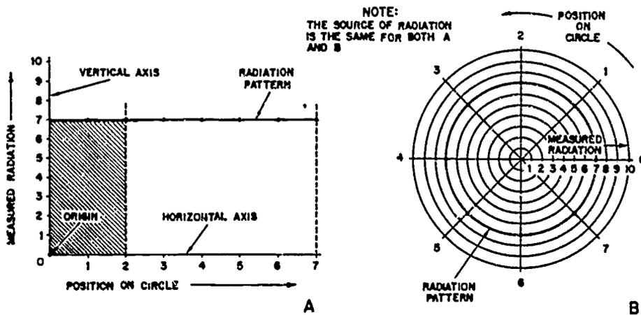
Fig 2-16. Comparison of rectangular- and polar-coordinate graphs for an isotropic source.
