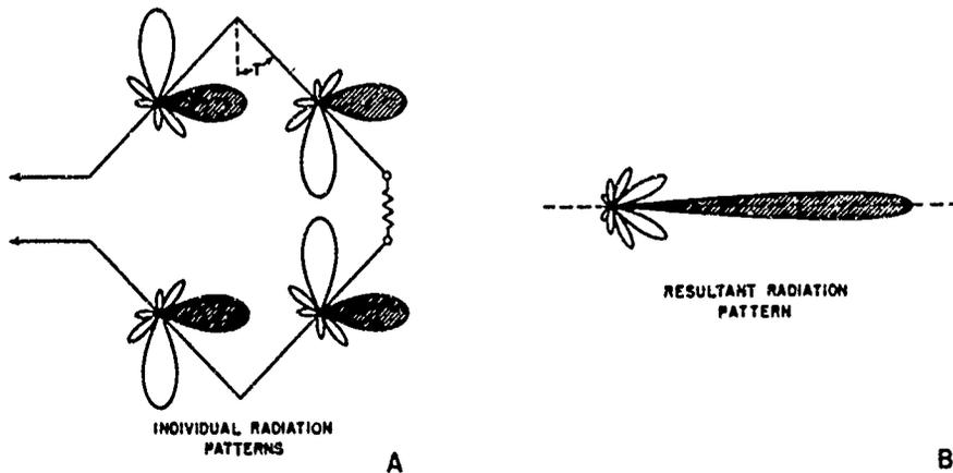
Fig 4-12. Formation of the rhombic radiation pattern.
