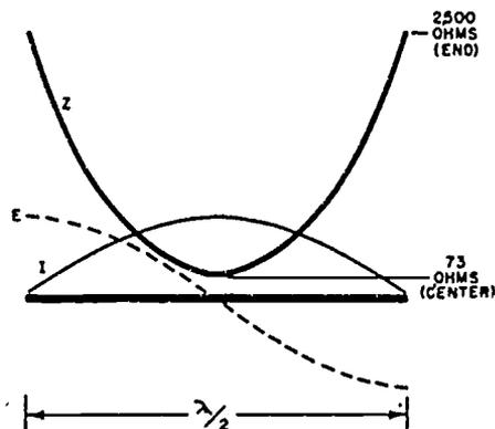
Fig 2-19. Impedance curve for a half-wave antenna.
