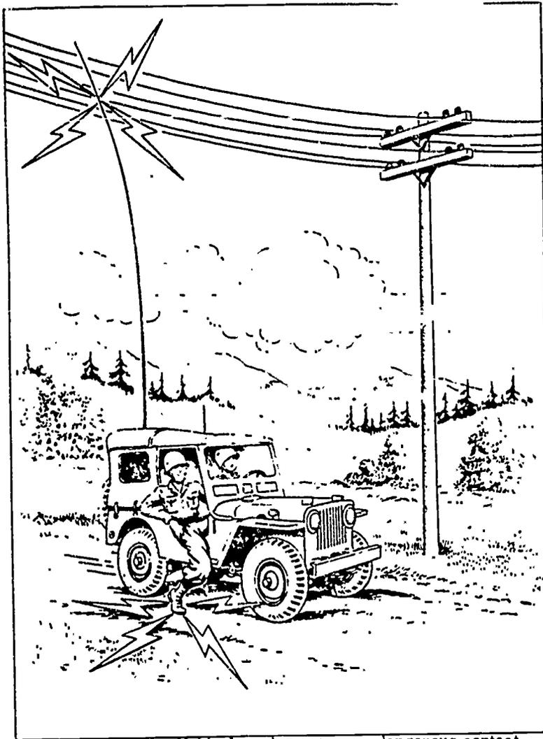
Fig 4-15. Vehicular whip antenna--dangerous contact.
