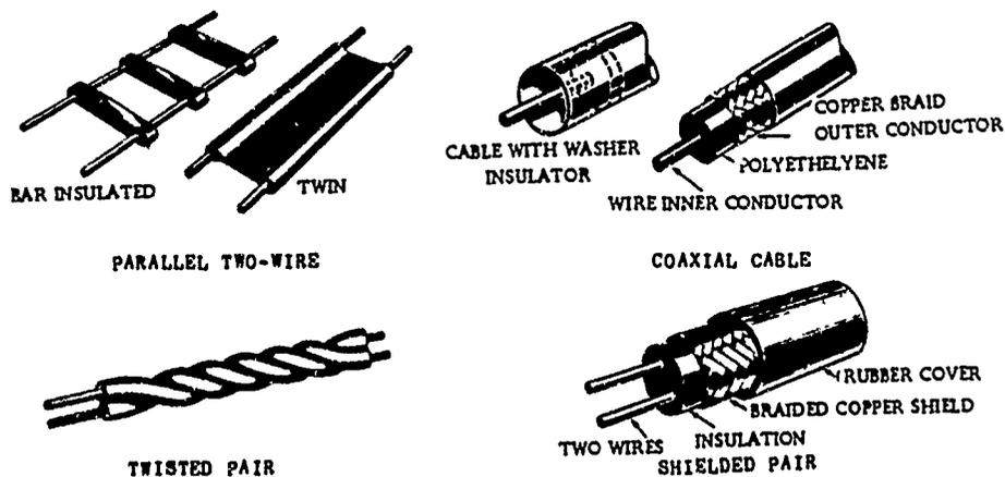
Fig 2-23. Four general types of transmission line.
