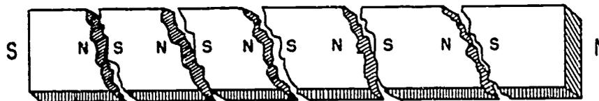
Fig 1-10. Magnetic poles in a broken magnet.
