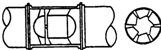
Figure 9. Vane axial fan.
