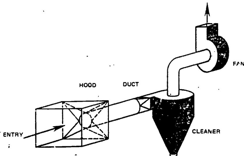
Figure 2. Elements of a local exhaust system.
