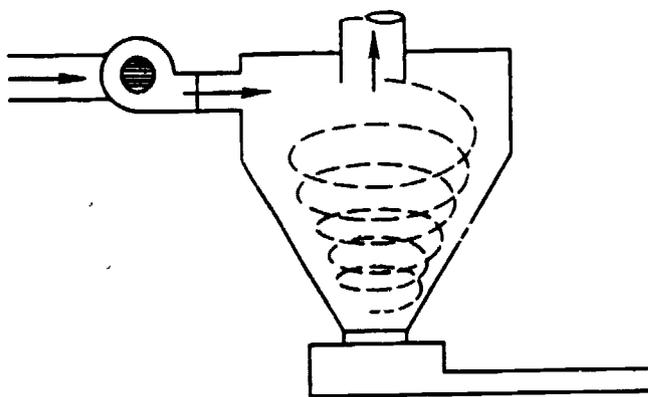
Figure 11. Cyclone collector.
