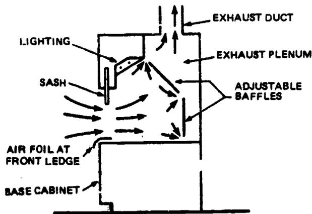
Figure 4. Standard laboratory fume hood.
