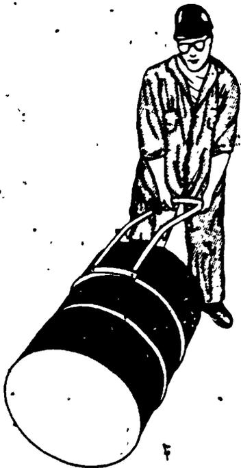
Figure 2. A lifter bar, or drum lifter.
