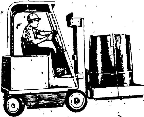
Figure 8. Industrial truck with platform.
