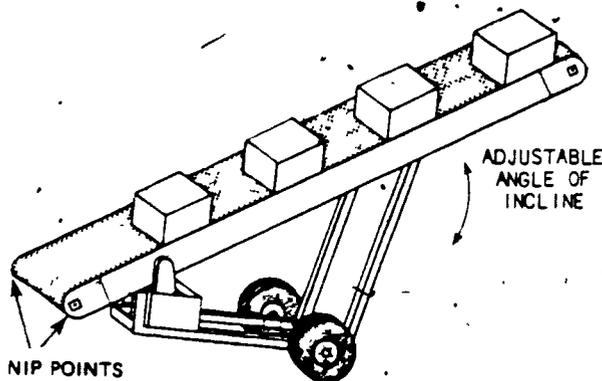
Figure 11: Powered portable belt conveyor.
