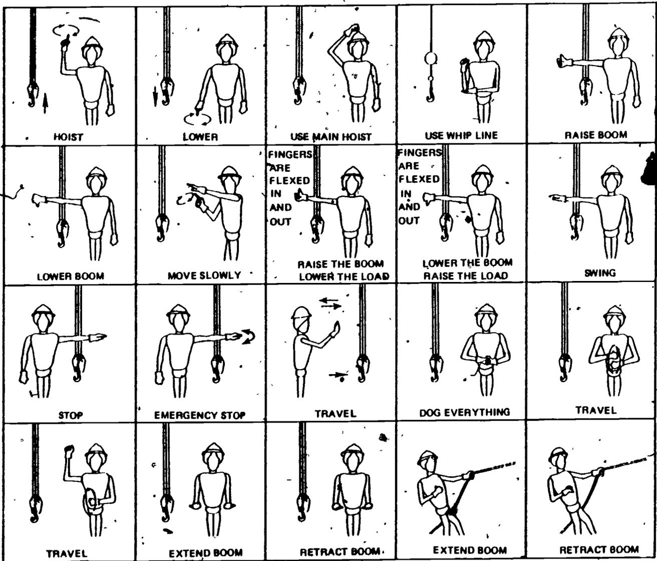
Figure 16.. Standard signals used in operating power cranes and shovels.
