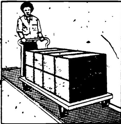
Figure 7. Four-wheeled hand truck.
